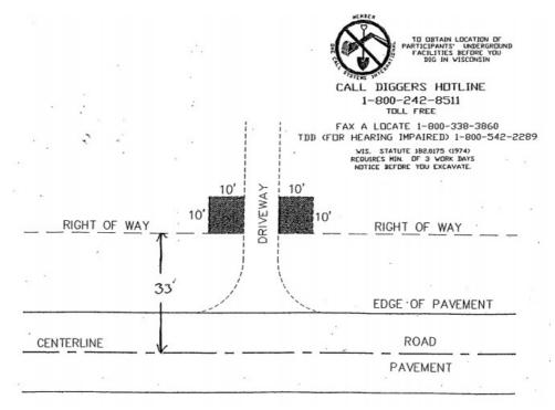
Post must be located in the shaded area on either side of the driveway.
